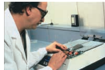
Figure 1: Table saw used to rough out component-mounted boards
