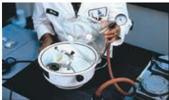
Figure 3: Vacuum impregnation equipment.
