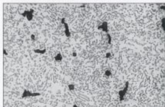
Fig. 4 — Spheroidize annealed O6 graphitic tool steel prepared with the H-RGD, see Table 2. Note the perfect graphite retention and the mixture of spheroidized and partially lamellar cementite in the ferrite matrix. (1000X, 4% picral etch).
