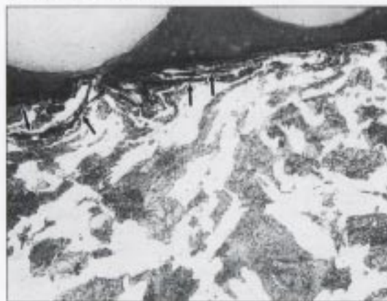
Fig. 1 — Surface of forged and annealed 5140 alloy steel exhibits surface cracks (arrows) using Flat Edge Filler shot in an epoxy mount for edge retention. (1000X, 4% picral etch).
