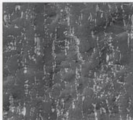
Fig. 9 — Microstructure of an annealed dual phase stainless steel (ferrite darkened) prepared according to Table 4, but with 6- \mu m diamond for step two, viewed with differential interference illumination mode. (200X, 20% NaOH at 1.5 V dc).
