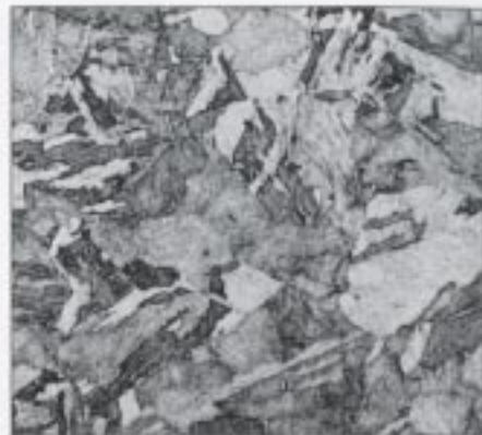
Fig. 7 — Microstructure of solution annealed and aged 18Ni250 maraging steel prepared according to Table 4. (1000X, Fry's reagent).
