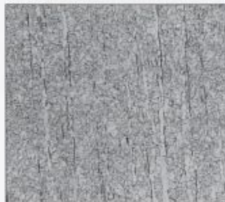
Fig. 8 — Microstructure of 416 free-machining stainless steel prepared according to Table 4, but with 6- \mu m diamond for step two. (200X, Vilella's reagent).
