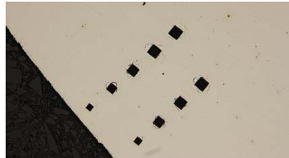
Figure 21: Vickers indents of a NHT measurement. The hardness decrease can be correlated with increasing indent size. Magnification 200x.
