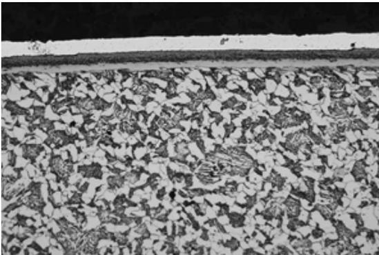
Figure 13: Nitrided layer after etching with 3% Nital. Magnification 200x.
