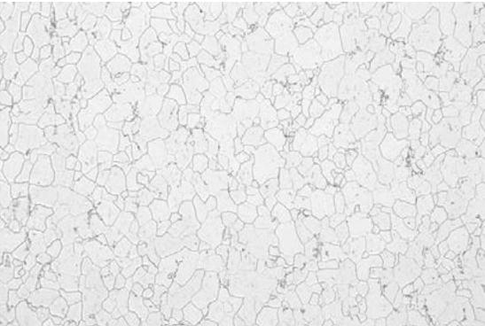
Figure 5: Soft iron, Ferrite grain boundaries with some nodular carbides. Etched with 3% Nital. Magnification 200x.
