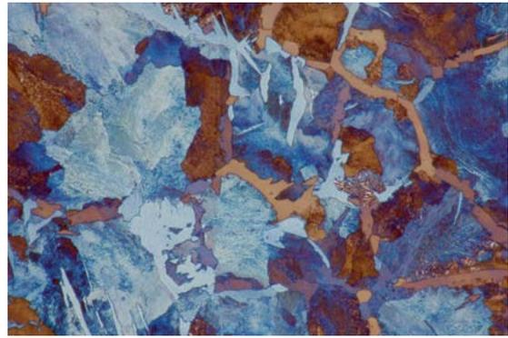
Figure 8: Normalized steel C35/1035, lamellar Perlite with Ferrite. Etched with Klemm I. Magnification 500x viewed with polarized light and sensitive tint..
