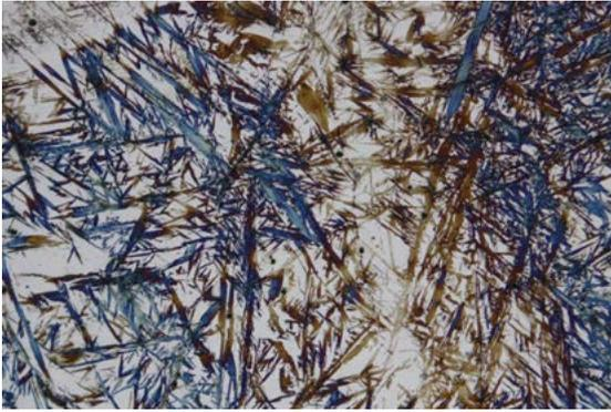
Figure 4: Martensitic Steel with retained austenite (white) etched with Klemm I. Magnification 200x viewed with polarized light and sensitive tint..
