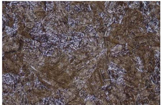
Figure 18: Martensite revealed with 3% Nital. Magnification 200x.
