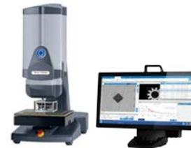
Figure 20: Wilson VH3300 automated Vickers hardness tester.
