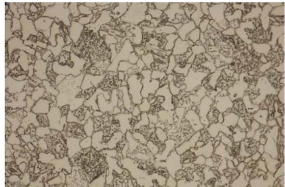
Figure 10: Spheroidised steel C45/1045, Ferrite grains and nodular Cementite. Etched with 3% Nital. Magnification 500x.
