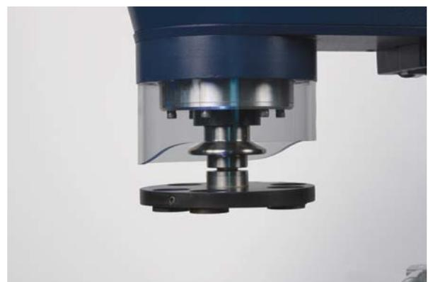
**Figure 3: Samples are clamped and aligned in a central force specimen holder.**
