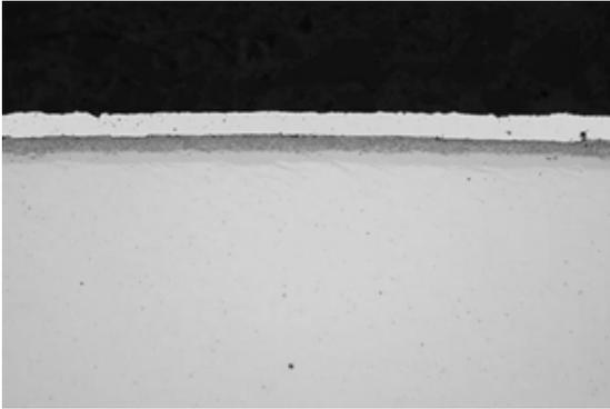
Figure 12: Nitrided layer, plated with aluminum foil. The porous layer inside the compound layer is well visible. Magnification 200x.
