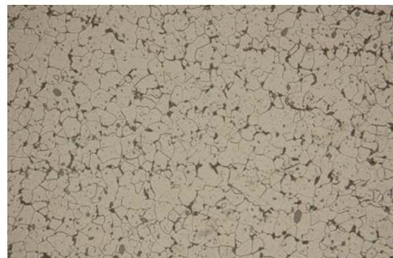
Figure 11: Machining steel 95Mn28K. MnS particles grey. Etched with 3% Nital. Magnification 200x.
