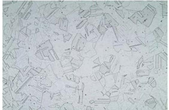
Figure 16: Stainless steel X5CrNi18-10. Etched with V2A at 60°C. Magnification 200x.
