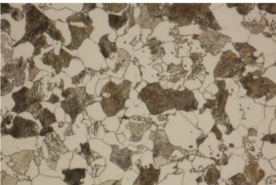
Figure 7: Normalized steel C35/1035, lamellar Perlite with Ferrite. Etched with 3% Nital. Magnification 500x.
