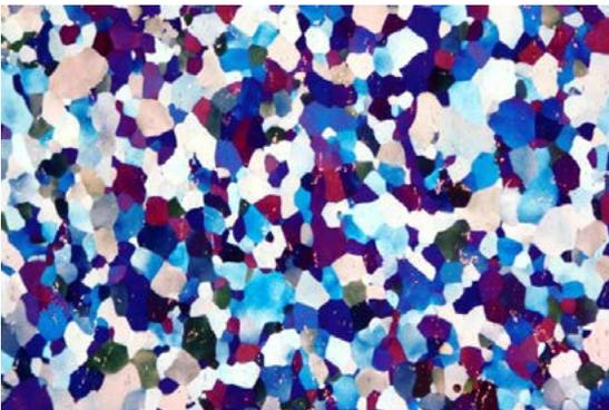
Figure 6: Soft iron, ferrite grains colored with Klemm I etchant. Magnification 200x viewed with polarized light and sensitive tint..
