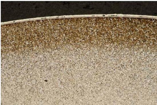
Figure 14: Nitrided layer. Diffusion zone after etching with 3% Nital. Magnification 100x.
