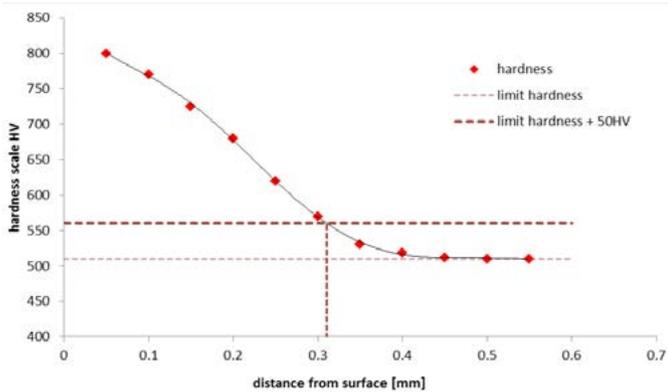
Figure 19: Principle of the NHD evaluation. Hardness is measured from surface to core, leading to a decrease in hardness for surface hardened materials.
