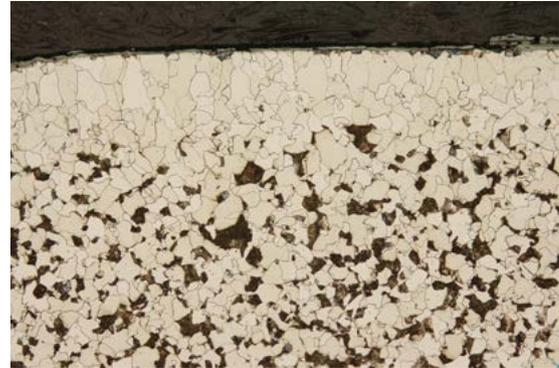
Figure 9: Heat-treated steel C45, hardened, surface decarburization. Etched with 3% Nital. Magnification 200x.
