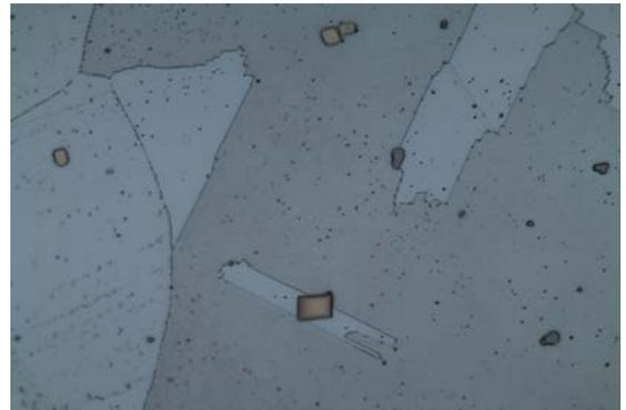
Figure 17: Stainless steel X5CrNi18-10. Ti (C,N) particles (orange). Magnification 1000x.
