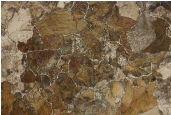
Figure 15: High-grade steel C100. Etched with 3% Nital. Magnification 500x.
