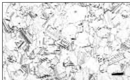
Fig 3 Material in Fig. 1 after solution annealing at 1010°C; acetic glycerregia etch; magnification bar is 100 \mu\text{m} long
