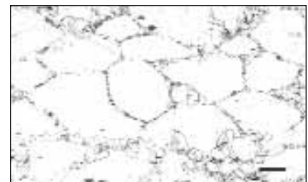
Fig 4 Necklace-type duplex grain structure in as-forged experimental 625-type alloy; acetic glycerregia etch; magnification bar is 100 \mu\text{m} long
