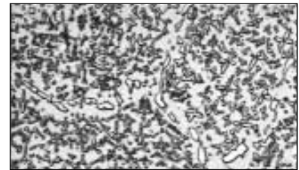
Fig 15 Coarse gamma prime in as-hot isostatically pressed René 95; glyceresia etch; magnification bar is 10 µm long
