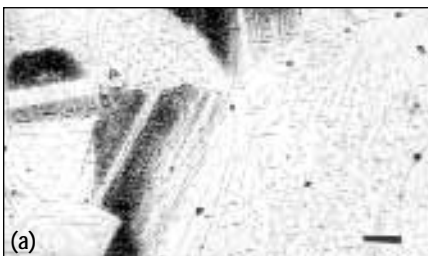
Fig 8 Precipitation of intergranular \eta phase in Pyromet 31 after 1,500 hours at 816^\circ\text{C} (a); glyceresia; magnification bar is 25 \mu\text{m} long (Note the grain boundary carbides); \eta phase in a Pyromet 31 specimen solution annealed at 954^\circ\text{C} (b); glyceresia etch; magnification bar is 10 \mu\text{m} long
