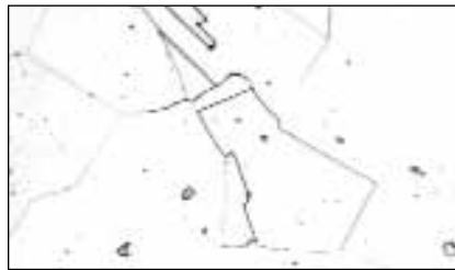
Fig 14 Normal solution annealed austenitic grain structure of Alloy 718 solution annealed at 1066°C (80 HRB); glyceresia; magnification bar is 100 µm long
