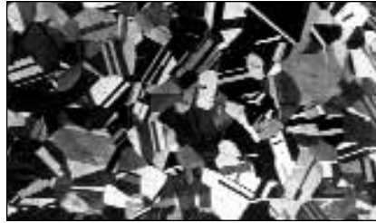
Fig 11 Fully recrystallized austenitic grain structure of Waspaloy solution annealed at 1066°C; modified Beraha's tint etch; magnification bar is 100 µm long
