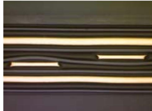
*Four layer, bi-directional flex circuit cross-section. 50x magnification.*
