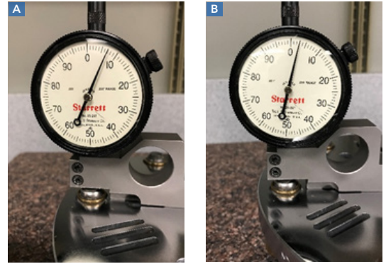
Figure 4: Setting the position for (a) diamond 'Long Stop' and (b) diamond 'Short Stop'
