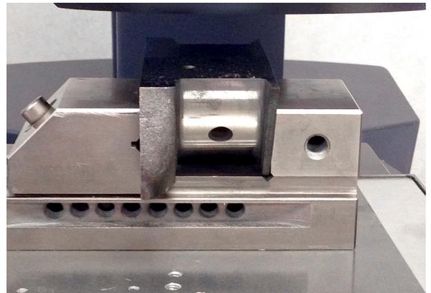
Figure 1.1 - Crank pin held in machinist vice
