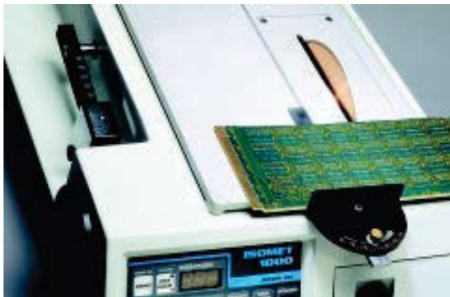
Figure 1. Figure 2. IsoMet® 1000 Precision Sectioning Saw with Table Saw accessory effectively sections or trims printed circuit boards
