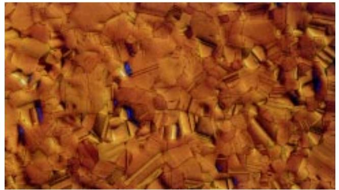
*Fig. 2 - Annealed cartridge brass prepared by the traditional method, followed by vibratory polishing with an attack polish agent in colloidal silica with multiple etch-polish cycles. This yielded a scratch free surface by excessive relief (Klemm's I reagent, 20X, DIC.)*
