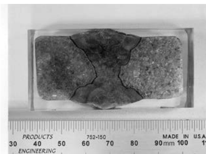
Figure 3. Large welds can be encapsulated in epoxy using rectangular molds.
