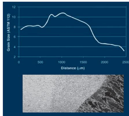
Figure 2. A cross section of a low carbon steel weld where the base metal is on the far left and the weld material is on the right. The grain size in the HAZ has been refined during the welding process.
