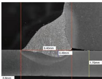
Figure 1. Operator interactive measurements of the weld leg (red), penetration (blue) and plate thickness (yellow) using the parallel and point-to-point tools for a low-carbon steel lap weld.
