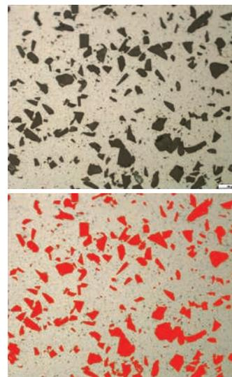
Figure 4. The silicon carbide particles in the Al-matrix (top) have been detected and highlighted with the red bitplane (bottom).
