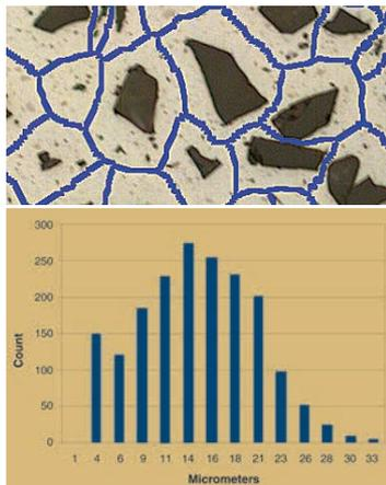
Figure 5. (top) A close-up of the blue cell outlines which resulted from expanding the SiC particles. Figure 6. (bottom) Histogram displaying the distribution of the center-to-center distances of the SiC particles.
