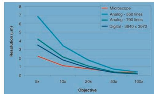
Figure 7. A comparison of theoretical resolutions is shown for three cameras and a microscope.
