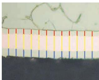
Figure 3. The thicknesses of the coin plating layers were evaluated by measuring the corresponding chords: Ni-red, Cu-yellow and Ni-blue.
