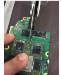
Figure 1. Illustrating sectioning of PCBA with the aid of table saw attachment on IsoMet 1000
