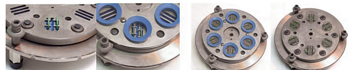
Figure 3. illustrating PWB met with PCB coupons mounted for targeted vias assessment
