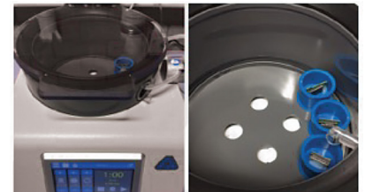
Figure 2. Illustrating SimpliVac mounting system for PCBAs or PCB samples
