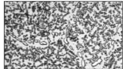
Fig 15 Coarse gamma prime in as-hot isostatically pressed René 95; glyceresia etch; magnification bar is 10  $\mu\text{m}$  long
