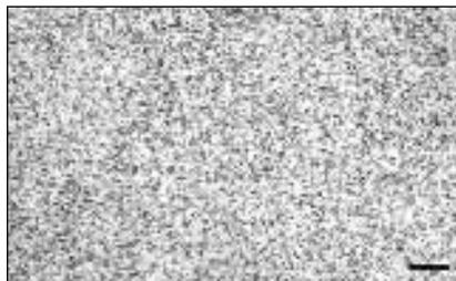
Fig 1 As-hot rolled grain structure of CustomAge 625 Plus, finish rolled at 1007°C; acetic glycerregia etch; magnification bar is 100  $\mu\text{m}$  long
