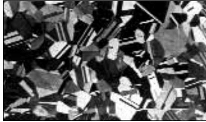
Fig 11 Fully recrystallized austenitic grain structure of Waspaloy solution annealed at 1066°C; modified Beraha's tint etch; magnification bar is 100  $\mu\text{m}$  long
