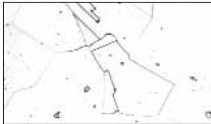
Fig 14 Normal solution annealed austenitic grain structure of Alloy 718 solution annealed at 1066°C (80 HRB); glyceresia; magnification bar is 100  $\mu\text{m}$  long
