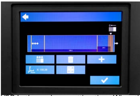
Figure 2. Serial Cut Programming to automatically cut the four locations.
