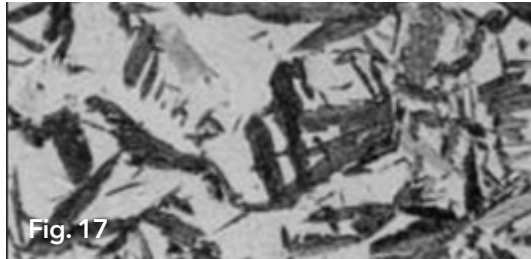
Figure 16. Upper bainite (dark) and martensite (light background) in a partially transformed (830 °C – 30 min, 538 °C for 1 min, water quench) specimen of 5160 alloy steel. The austenite not transformed to upper bainite after 1 minute formed martensite in the quench (2% nital, 1000x). Figure 17. Lower bainite (dark) and martensite (light) in a partially transformed (830 °C – 30 min, 343 °C for 5 min, water quench) specimen of 5160 alloy steel. The austenite not transformed to lower bainite after 5 minute formed martensite in the quench (2% nital, 1000x).
