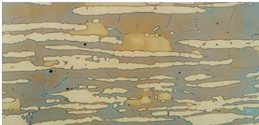
Figure 6. Ferrite (colored) and austenite (white) in 2205 duplex stainless steel electrolytically etched with aqueous 20% NaOH, 3 V dc, 10 s (100x).
