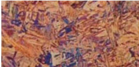
Figure 18. Lath martensite in quenched and tempered 4118 alloy steel revealed by etching with Beraha's sulfuric acid etch, (500x).
