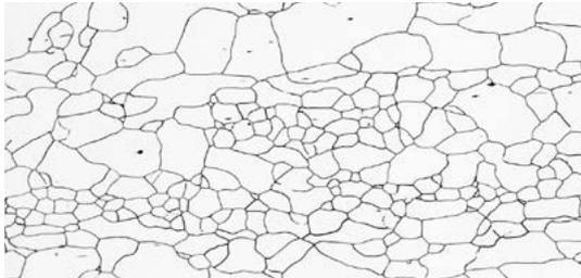
Figure 2. Ferrite grain structure of a ferritic stainless steel (Fe - <0.01% C - 26% Cr - 1.2% Mo - 0.035% Nb - <0.015% N) electrolytically etched with aqueous 60% nitric acid, 1.2 V dc, 15 s (100x).
