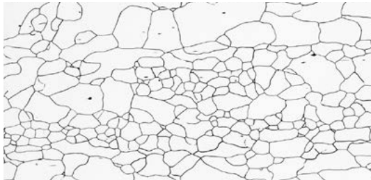
Figure 2. Ferrite grain structure of a ferritic stainless steel (Fe - <0.01% C - 26% Cr - 1.2% Mo - 0.035% Nb - <0.015% N) electrolytically etched with aqueous 60% nitric acid, 1.2 V dc, 15 s (100x).
