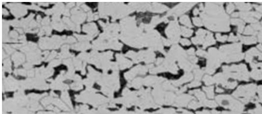
Figure 13. Microstructure of plate steel from the RMS Nomadic containing proeutectoid ferrite (white) and pearlite (dark) revealed by etching with 2% nital (200x).
