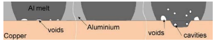
Figure 3. Schematic of Al-Cu weld highlight features expected when Al melts and Cu remains in solid state (Zwicker 2020)
