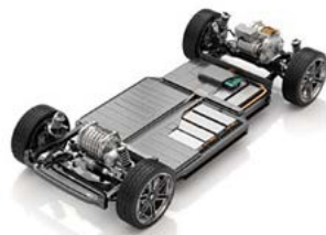
Figure 2. a BEV platform system
