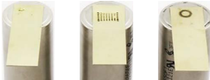
Resistance spot welding (RSW)
