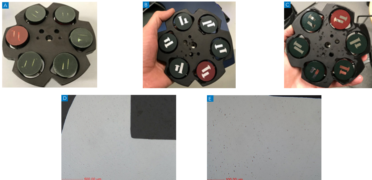
Figure 9. (a) before planar grinding (b) ground to centre of samples (c) after first polishing step (d) head and radius showing good edge retention (e) polished surface at (20x) magnification
