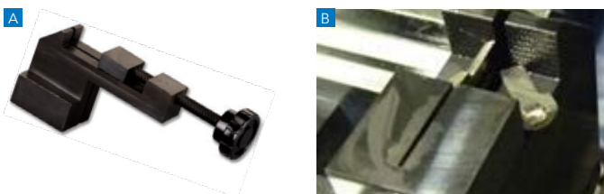
Figure 5. (a) showing a fastener chuck, and (b) showing fastener sectioning using the chuck on an abrasive cutter
