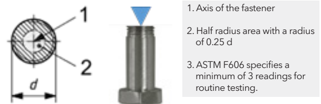
Figure 2. cross section hardness indentation
