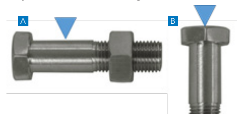
Figure 3. (a) unthreaded shank, (b) head region
