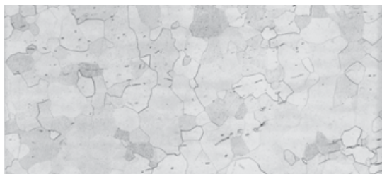
Figure 8. Annealed CP Ti (ASTM F67, Grade 2) after using 0.05µm alumina in step 3, with the attack polishing agent (200x, Kroll's reagent).
