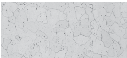
Figure 7. Best results obtained for annealed CP Ti (ASTM F67, Grade 2) using the 3-step method of Müller (200x, Kroll's reagent).
