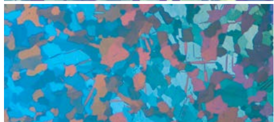
Figure 9. As-polished CP Ti (as hot rolled) viewed with crossed polarized light (100x). Figure 10. The same specimen as in Figure 9, but after 2h vibratory polishing (100x, crossed polarized light).
