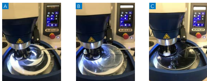
Figure 4. (a) just before last 20seconds (b) flushing surface with water, and (c) last 2-3 seconds
