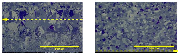
(a) Deformation induced by incorrect cutting
