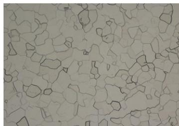
Contrasting of the titanium grade 2 sample with Kroll's etchant.
