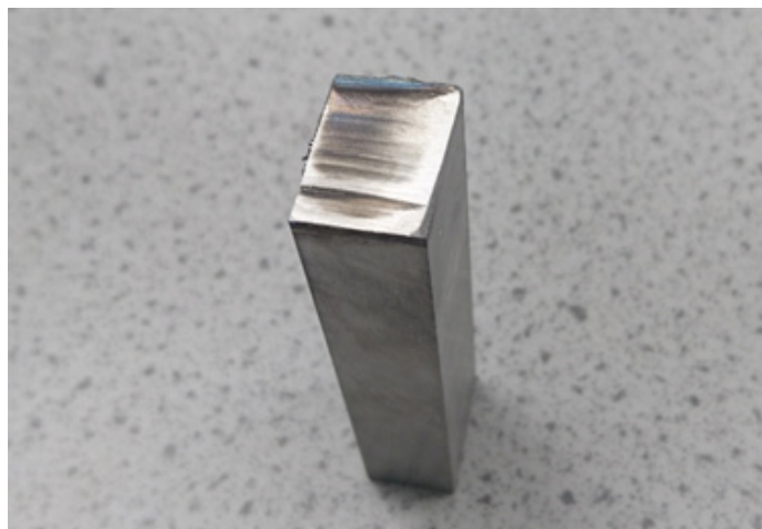
Figure 1. Tarnishing of a titanium sample due to incorrect selection of the cutting disc and insufficient cooling during the cutting process.
