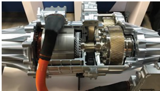
Figure 1. Showing an example of an EV powertrain for heavy duty trucks ~ Courtesy of Magna
