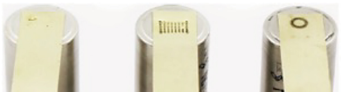
Figure 5. Illustrate welds tests on a lithium batteries with left - spot weld, middle - ultrasonic weld and right laser weld
