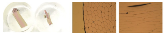
Figure 5. Illustrates example of a crimped connector with cross-sectional and longitudinal views
