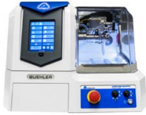
Figure 1: Isomet High Speed saw - used at 4000rpm and 3mm/min cut speed with an Isocut HC blade
