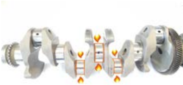
Figure 1.1 Shows a crankshaft with illustration of induction heating of the surface layer of the crank journals
