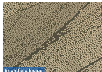
Figure 3 showing surface finish after 0.05µm alumina on Microcloth prepared by manual preparation.
