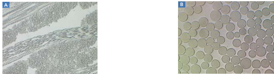
Figure 4 (a) low magnification and (b) high magnification showing glass fiber reinforced composite (GFRP) after 0.05 \mu\text{m} alumina polishing on Microcloth prepared semi-automatically on a grinder polisher.
