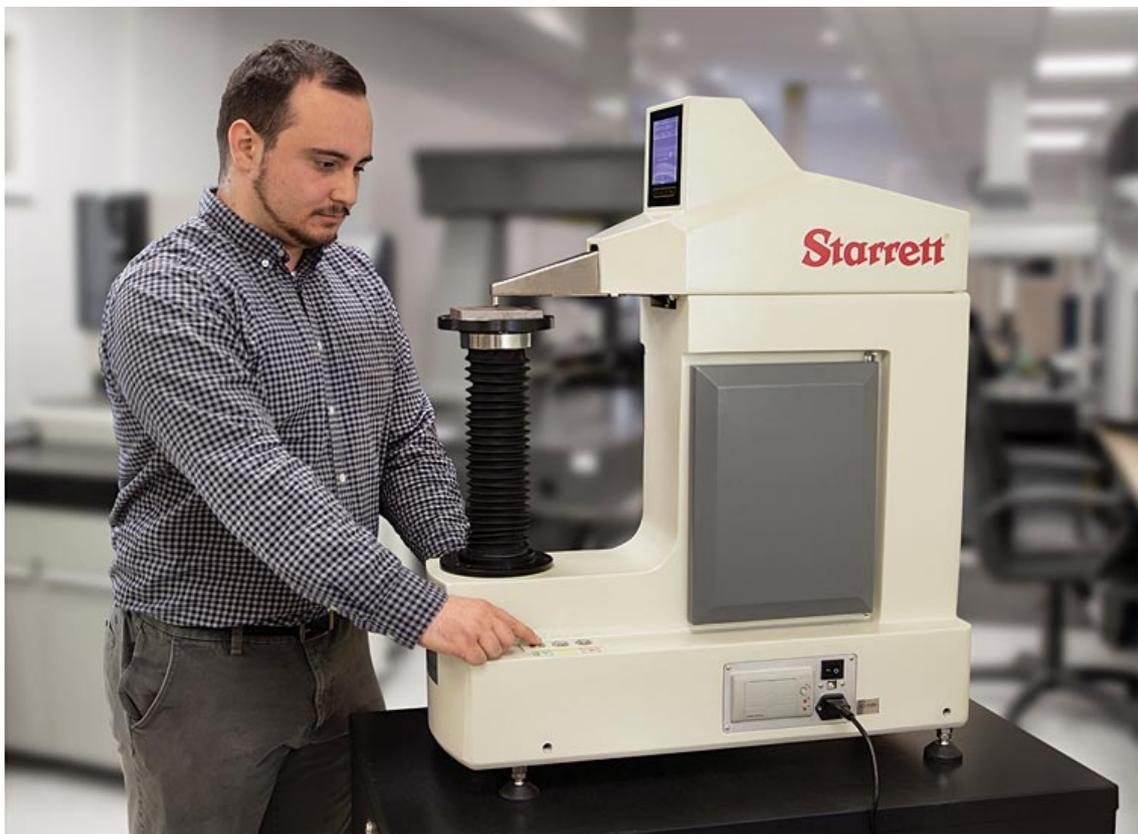
*An operator stands next to the new Starrett Digital Rockwell/ Superficial Rockwell Benchtop hardness tester No.3824 with fully automated load/ unload procedures, and capable of providing highly accurate readings.*
