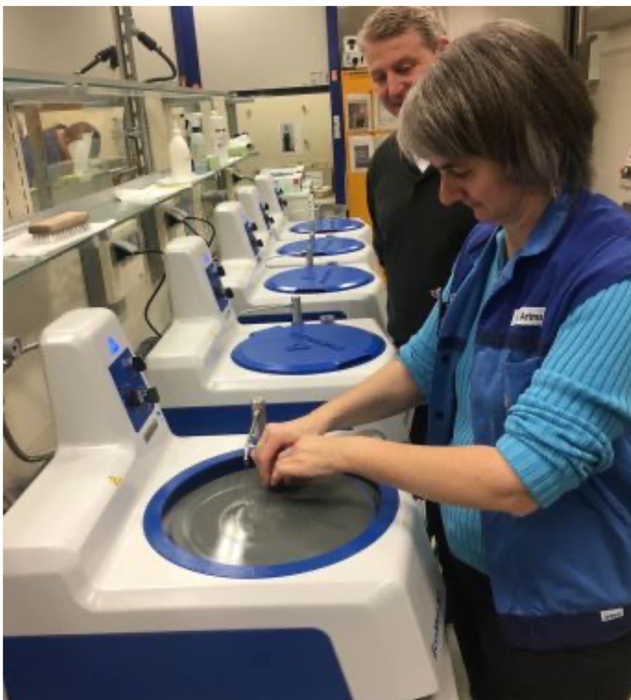
In addition to the single platen models now in service at BMW, EcoMet 30 grinder-polishers are also available in a twin platen version. Both models are offered for manual or semiautomatic operation.
