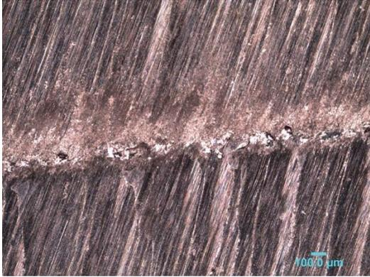
Figure 2 At the interface with the coating, material has been heavily damaged and fallen out requiring extended grinding and polishing to recover.
