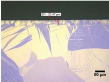
Precision blade recrystallization at 20µm shows minimal twinning.
