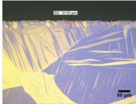
Abrasive wheel recrystallization at 30µm shows some mechanical twinning.
