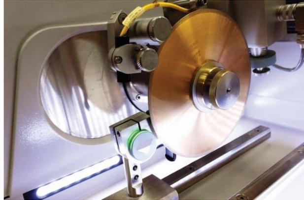
*Figure 4 The goal with precision cutting is to minimize damage to the sample and to maximize the amount of flawless surface available for analysis.*
