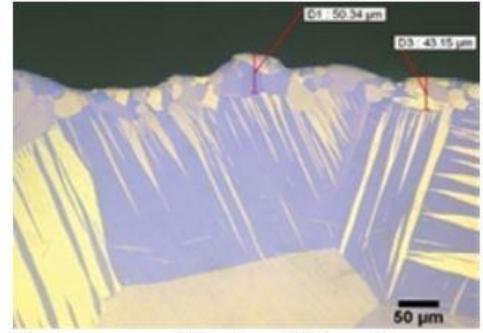
Band saw recrystallization at 50µm shows jagged edges and heavy mechanical twinning that could prolong grinding time.
