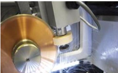
Figure 3 Automatic dressing, periodically during the cut, improves, speed, quality and consistency.
