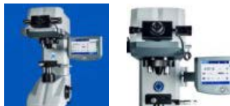
The Wilson VH1202 universal micro-hardness tester features deadweight loads from 10 g up to 2 kg and nine different, automatically selectable loading stages. It is equipped with a six-position turret, including two indenters for both Knoop and Vickers, and an additional objective with 5X magnification at long working distance. (Photo courtesy of PRNewsFoto/Buehler)
