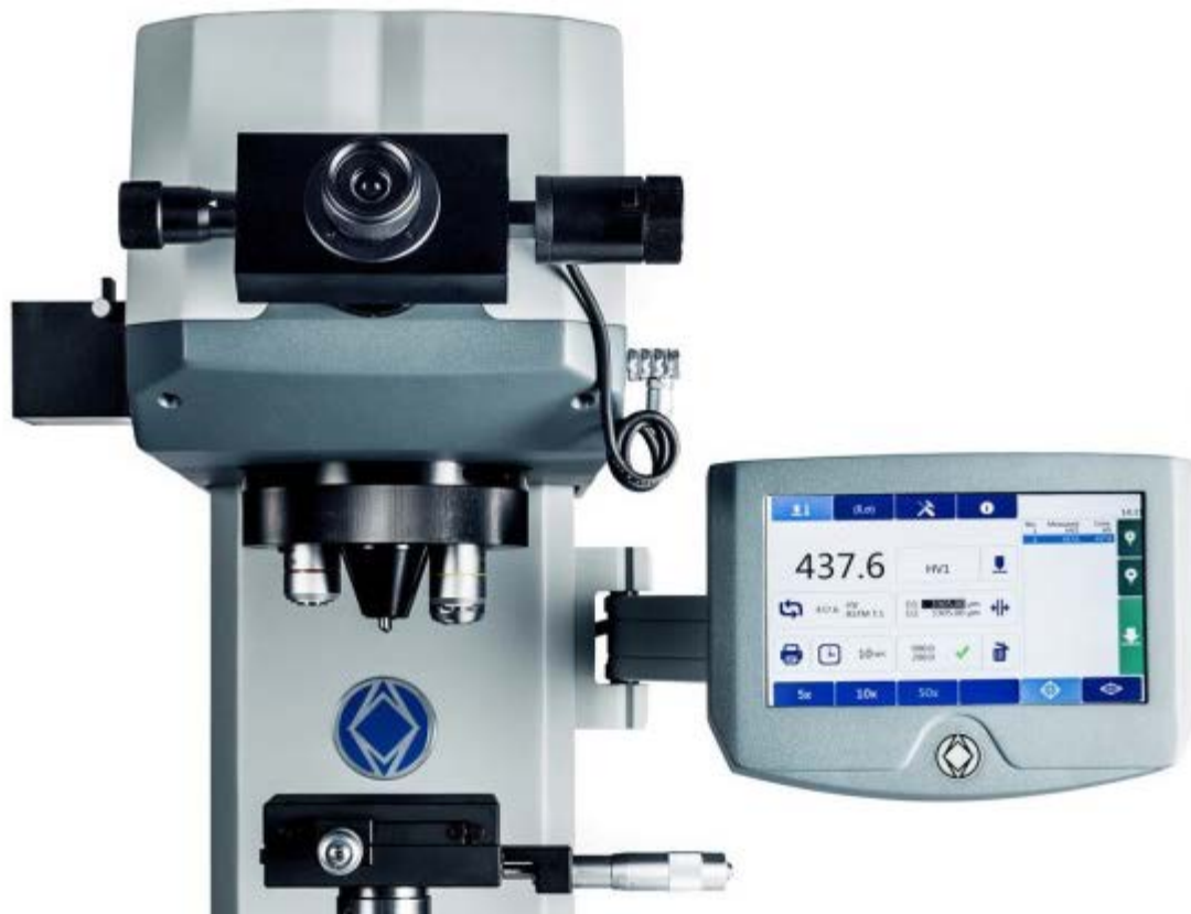
The Wilson VH1102 universal hardness tester.
