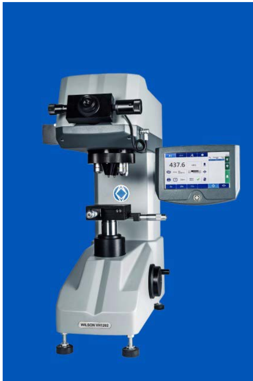
The Wilson VH1202 universal hardness tester.
