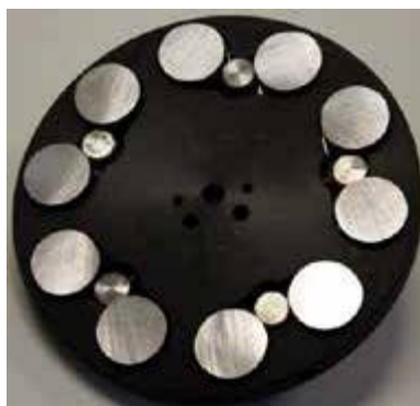
Figure 1. Unmounted bar material clamped in a central force 1.25 in [32 mm] specimen holder
