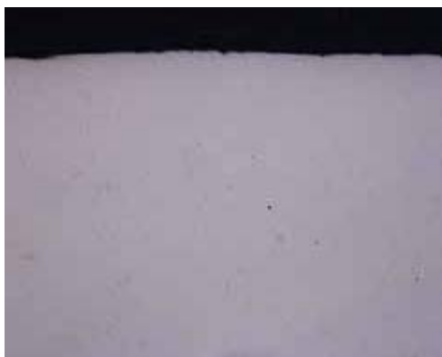
Figure 3. Surface quality after polishing on MicroFloc with 3 μm MetaDi diamond suspension. Magnification 200x
