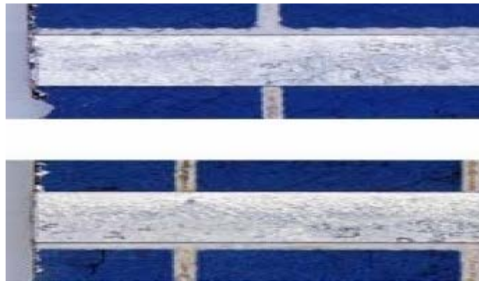
Figure 2. Interconnector on a soldered solar cell sample exhibiting a poor quality cut (top) and a good quality cut (bottom)
