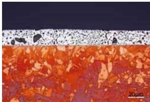
Figure 18. Sn62-Pb36-Ag02, etched with Klemm II, Eutectic solder material with Pb-rich solid solution (dark) and Sn-rich solid solution (light-colored)
