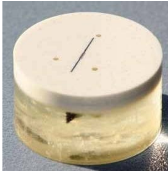
Figure 8. Solar cell with interconnector held perpendicular to the cross section with a UniClip Support Clip before epoxy mounting.
