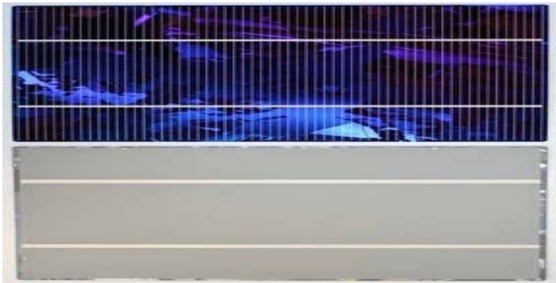
Figure 4. Front side, top and back side of a polycrystalline Silicon solar cell
