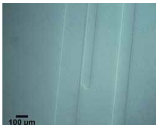
Figure 20. High purity, defect-free, polycrystalline silicon viewed with Nomarski DIC (etched with 100mL water, 75g NaOH)
