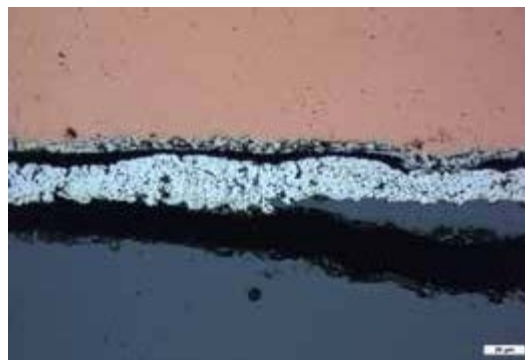
Figure 16. Light optical images showing delamination of a contacted bus bar at the cell interconnect and cracking seen across the wafer in dark gray at the bottom
