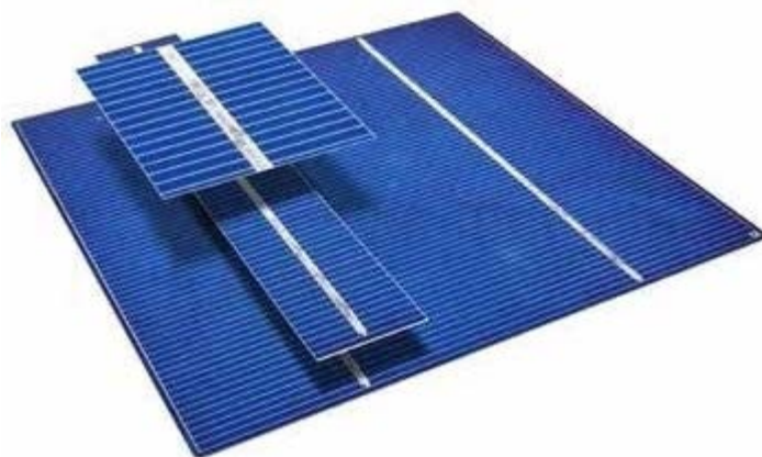
Figure 6. Sectioning of the bus bar into samples appropriate for mounting
