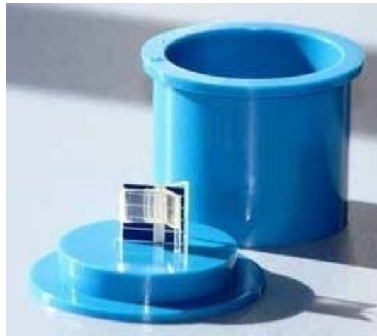
Figure 8. Solar cell with interconnector held perpendicular to the cross section with a UniClip Support Clip before epoxy mounting.
