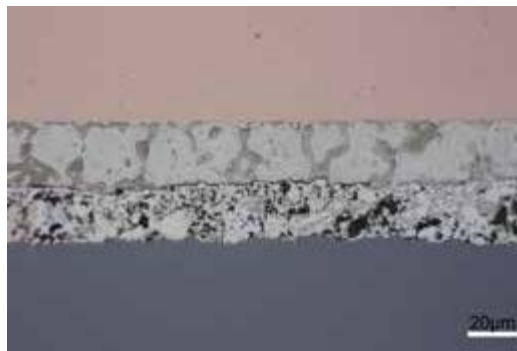
Figure 17. Microstructure of Bismuth containing lead-free solder Sn60-Bi38-Ag02 (unetched) interconnect
