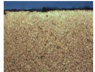
Martensitic structure with surface oxidation. Etched with Nital 3%, Magnification 200x
