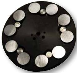
Unmounted bar material clamped in a central force 1.25in [32mm] specimen holder (60-5282)
