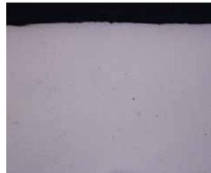
Surface quality after polishing on MicroFloc with 3µm MetaDi diamond suspension. Magnification 200x
