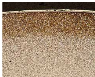
Nitrided layer. Diffusion zone after etching with 3% Nital. Magnification 100x.
