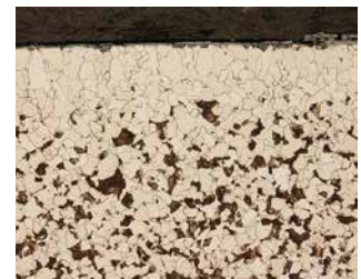
Heat treated steel C45, hardened, surface decarburisation. Etched with 3% Nital. Magnification 200x.
