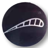
Airfoil mounted in EpoMet™ G.
