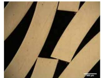
Surface finish after 9µm diamond polishing on UltraPad cloth at 50X.
