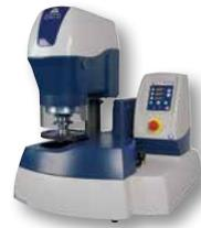
For a cycle time of 1min and 10sec, the average material removal was 300µm. For higher material removal rates, the cycle time was increased to 2min and 10sec. The average material removal achieved was 600µm.
