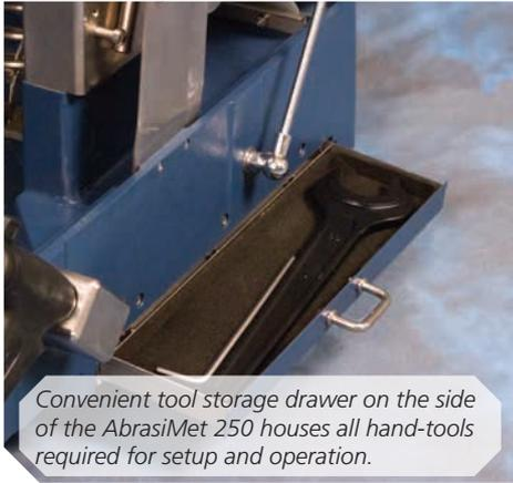
Convenient tool storage drawer on the side of the AbrasiMet 250 houses all hand-tools required for setup and operation.
