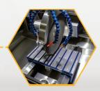
3 Axis Movement Provides flexibility and full range blade positioning allowing for the cutting of a variety of sample shapes and sizes
