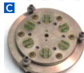
(a) Coupons mounted into holder prior to pouring the resin (b) cured mounts in the mounting assembly (c) the grinding fixture with the molding plate removed
