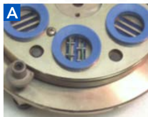
(a) Coupons mounted into holder prior to pouring the resin (b) cured mounts in the mounting assembly (c) the grinding fixture with the molding plate removed
