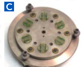
(a) Coupons mounted into holder prior to pouring the resin (b) cured mounts in the mounting assembly (c) the grinding fixture with the molding plate removed
