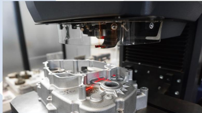
The target laser helps to position the part correctly on the big workpiece stage.
