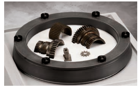
Large unmounted specimens may be polished with ease. Once loaded, specimens require little operator attention.
