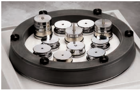
Generous specimen capacity allows up to 18 mounted specimens to be prepared simultaneously.
