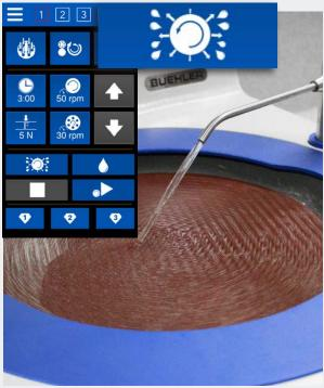
On the main screen, press and hold the "Rinse and Spin" button to begin the cycle.
