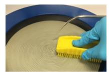
If material removal rates remain low after cleaning, dress the surface using a dressing stone. This will expose the cutting surface again and increase material removal rate.
