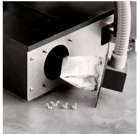
Vacuum system and dust collection bag.
