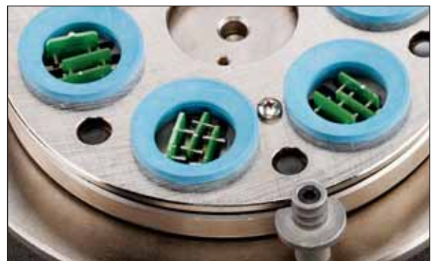
Printed wiring board coupons ready for molding compound in the PWB Met Small Hole Accessory.
