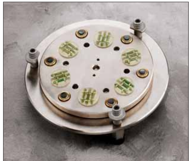
Mounted samples in the PWB Met® Small Hole Accessory.
