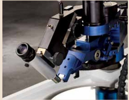
Bare die sample is easily aligned with the Tilt Cross-hair Alignment Microscope Accessory.
