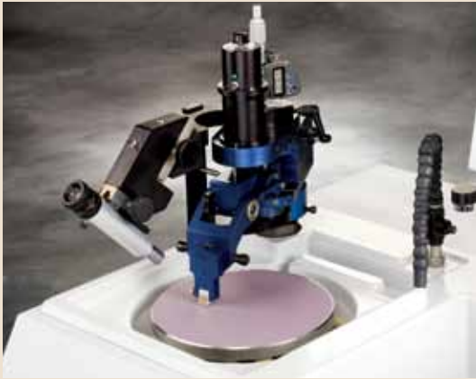
Bare die grinding on 1µm Diamond Lapping Film.
