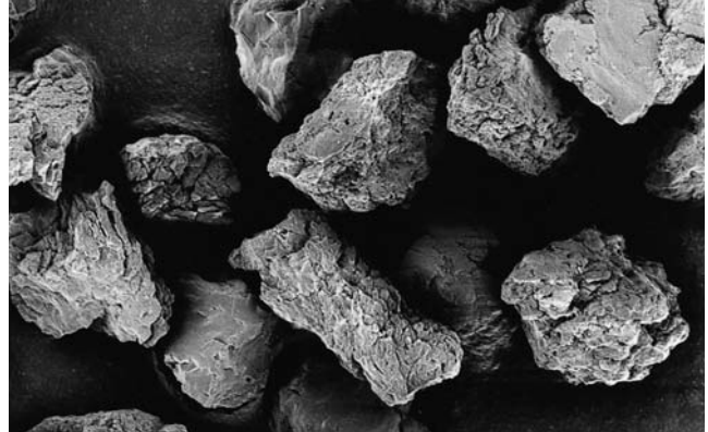
Angular, blocky-shaped polycrystalline diamonds of MetaDi® Supreme provide numerous cutting facets on the particle surface, resulting in less deformation.
