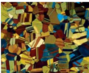
Left: Cartridge Brass, tint etched with Klemm's III, in cross polarized light with a sensitive tint filter. 50x. Right: Cartridge Brass indexed EBSD pattern. Quality Index: 221±8.6
