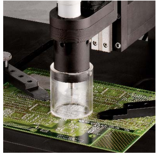
Printed wiring board clamped in router. A plastic safety shield directs cuttings into the vacuum dust collection system.
