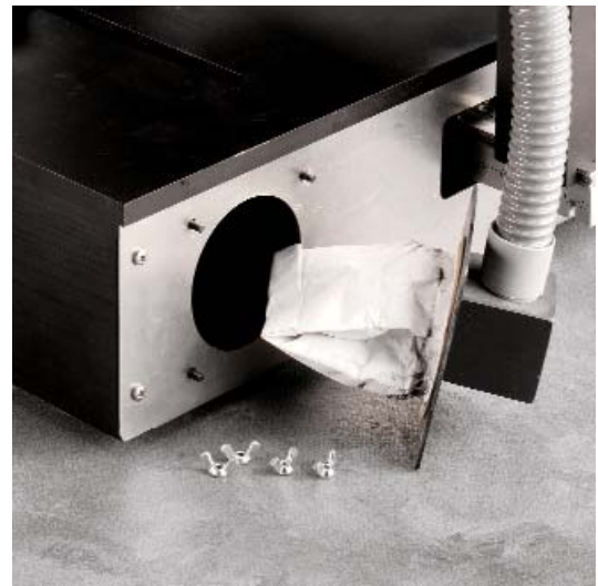
Vacuum system and dust collection bag.
